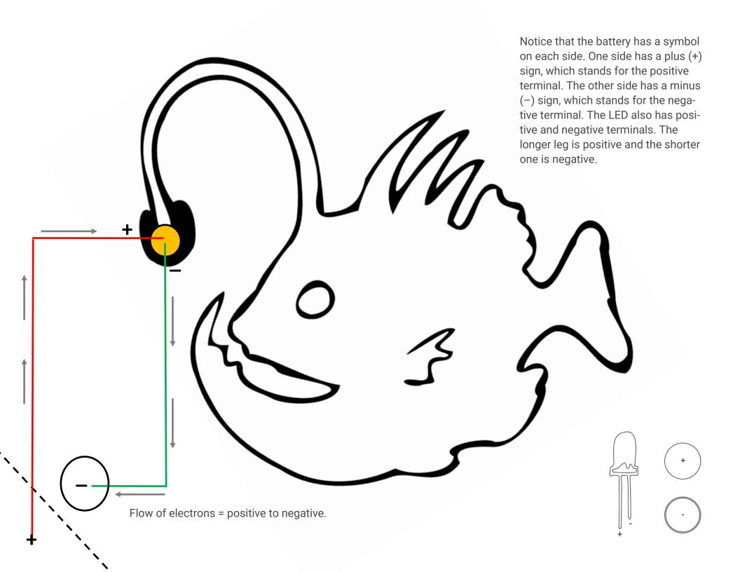
Basic circuit structure. An electrical circuit is a path on which electricity flows. Basic parts:
